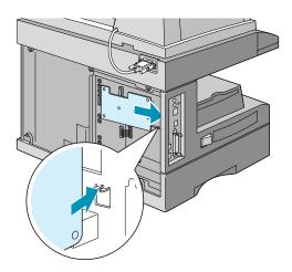
**10** Align the connector of the network interface card with the network card port on the control board and press the card until it is securely seated on the board.
